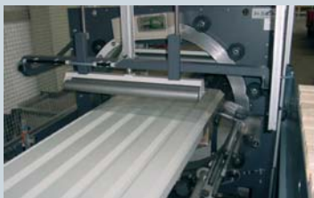
Automatic packaging for roof panels
