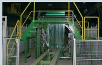
Inline solution for sandwich panels with 6-side packaging
