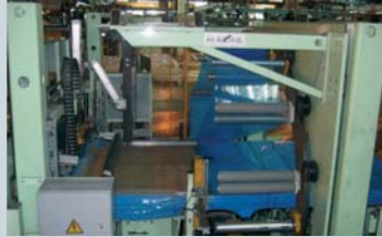
Wrapping with stretch film for mechanical and corrosion protection
